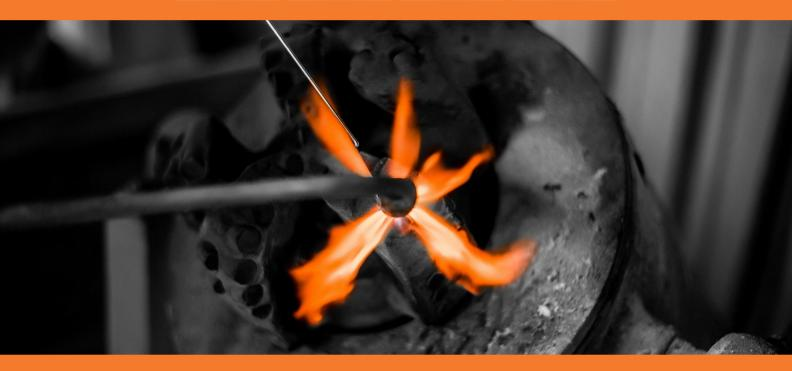
B it bodies are repaired and hard facing is applied during this stage. After the brazing, the bit is cooled before the next stage. This is step is mainly dealing with the body of the bit.
