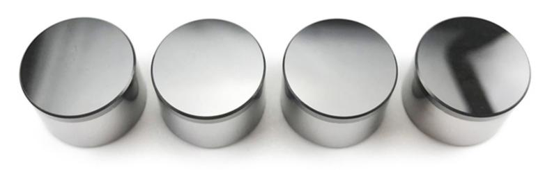
In this stage, we use selected cutters to replace old and worn cutters. The client has the option to use Premium, Premium Plus, or Standard cutters based on their requirements and application needs. Also, if there is any more modification needed to be applied on bits, it will be done. The procedure includes planning, components selection, and order from the warehouse.
