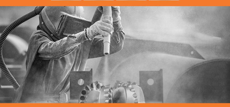
The next step of the cleaning process is blasting. Small particles using high air pressure remove the remaining dirt. All dirt for the cleaning process is collected, treated for re-use, or removed by specialized companies.
